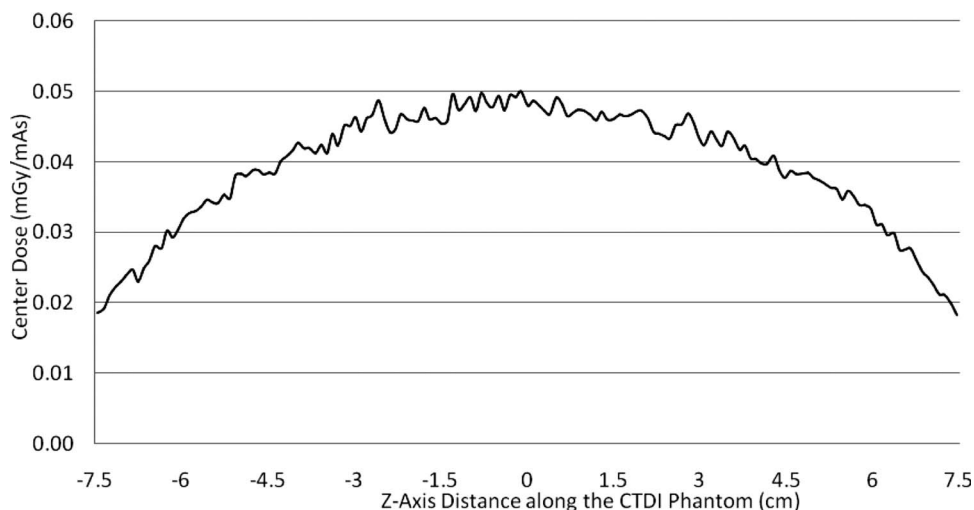
FIG. 1. Center dose profile for 32 cm CTDI phantom, pitch 1.0 helical scan, measured beam width 34.1 mm. All central profiles were similar due to the smoothing effect of the large scatter contribution at the center of a large phantom.
