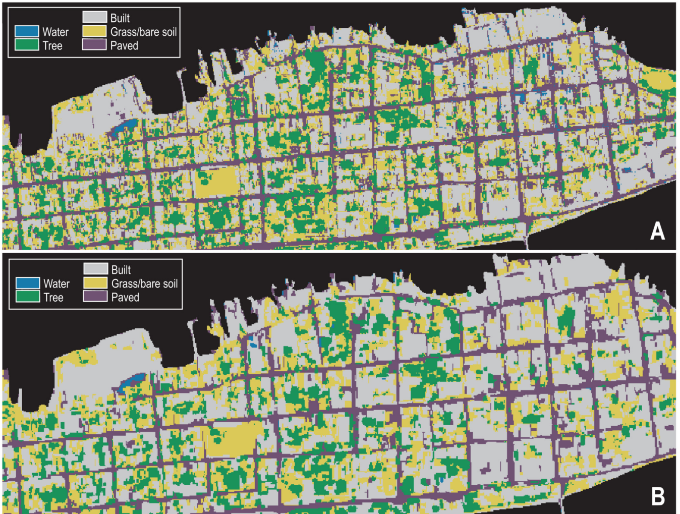
Figure 4. Masked sections of the back-propagation artificial neural network (A) and object-oriented classification (B) land use/cover maps of downtown Puntarenas, Costa Rica
