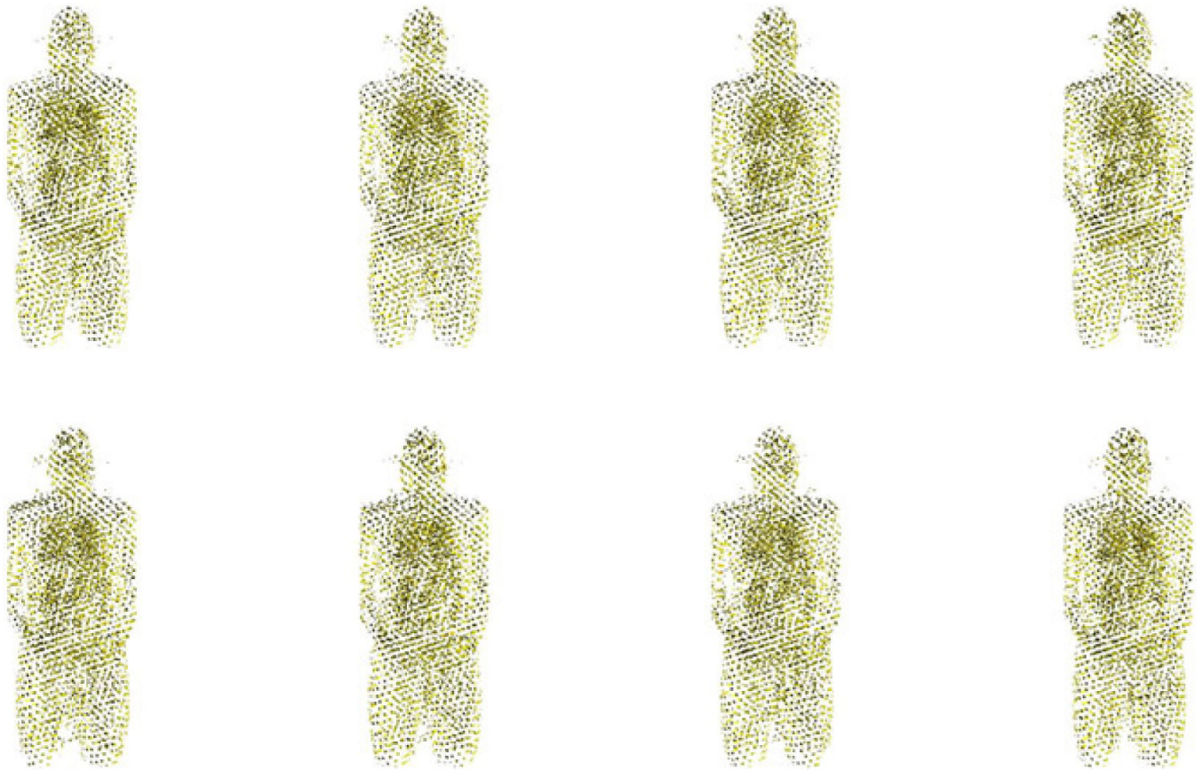
Fig. 11. Individual portions of an isosurface (isovalue = 800) extracted from the visible male MRI data with eight computing processors and rendered by the same set of machines. The full resolution isosurface has 9,128,798 triangles.
