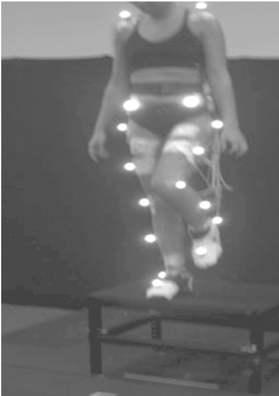
Figure 1. The 40-cm drop jump. Participants dropped single-legged from the platform onto the force plates. On landing on the force plate, participants performed a maximal vertical jump.
