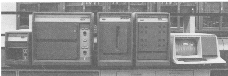
FIG. 1. AMS (left to right: diluent dispenser, filling module, reader-incubator, computer module, and data terminal).
