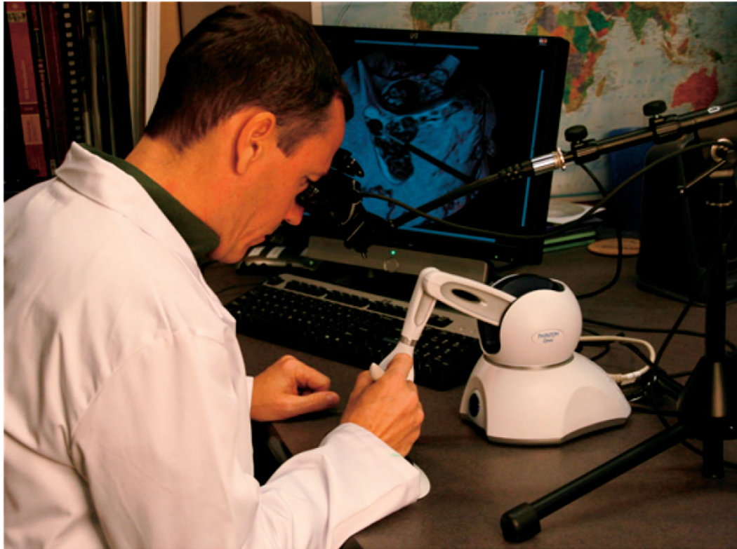
Fig. 3. A user running the full system, with a binocular display, haptic device, and speaker bar for outputting the sound of the drill.
