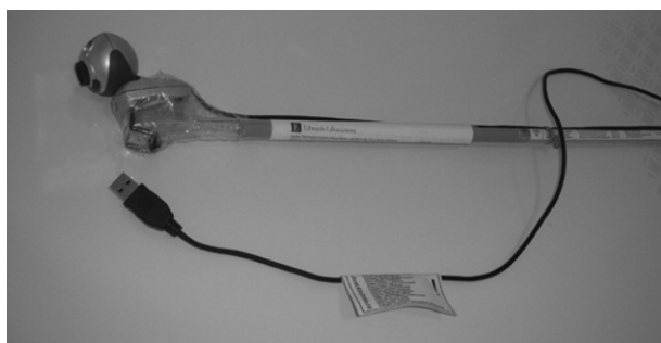
Figure 1 A webcam attached to outer plastic sheath of an embolectomy catheter.
