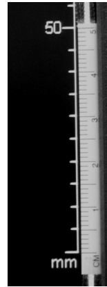
Figure 1 Calibration of image magnification using plastic ruler.
