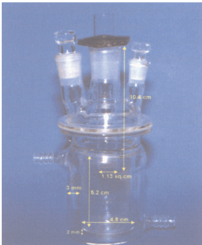
Figure 1. In vitro nasal diffusion cell (used with sheep nasal mucosa).
