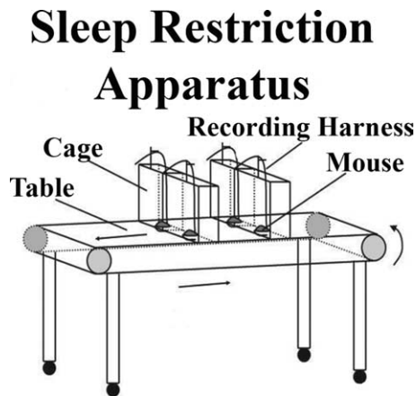
Figure 2. Sleep restriction apparatus. To sleep restrict mice, a 6 h cycle composed of 4 h of enforced waking and 2 h of uncontrolled behavioral state (4 h on and 2 h off) was used. Mice were placed in a Plexiglas cage with no bottom, 1/4 inch above a treadmill that moved at a speed of 3 cm/s. Food and water tubes were placed in each cage.
