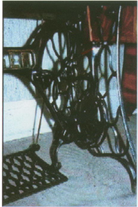
Figure 7. Understructure of the sewing machine. The sand-cast treadle and drive wheel, which also serves as main flywheel, have rough decoration; the functional features are mainly those of mass and strength. The open pattern of the treadle reduces the amount of material used and minimizes accumulation of dust and dirt.
