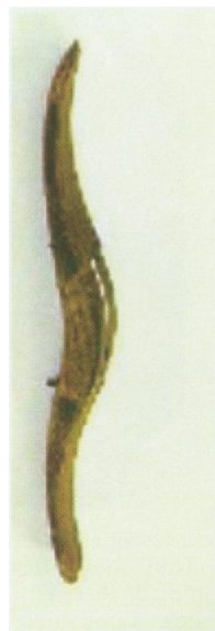
Figure 5. A crude antique shaving tool—uncomfortable to grip, and likely to chip and gouge the wood that it is used on.
