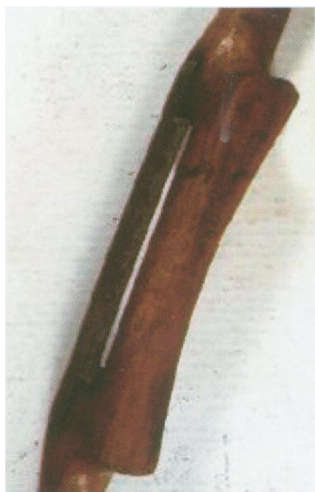
Figure 4. Underside of center portion of antique spoke-shave. The blade uses only a small piece of steel. The bearing surface, which slides along the work, is curved in such a way that the depth of cut can be adjusted simply via the angle at which the tool is held.
