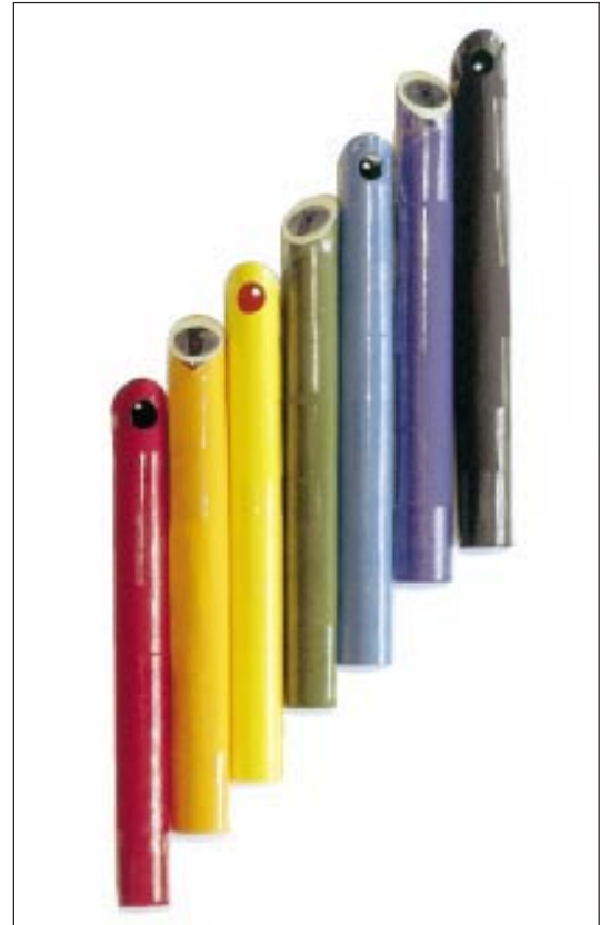
Fig 4 A spectrum of training ophthalmoscopes. A black lining is necessary with light-coloured instruments to prevent glow. Note black glare shields
