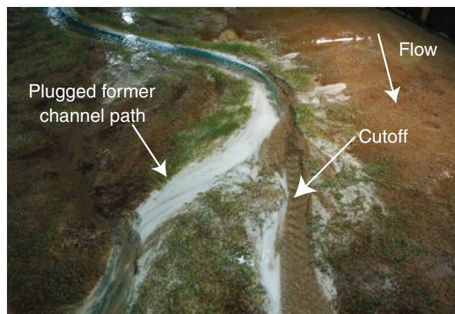
Fig. 5. Photograph of cutoff channel and fine sediment filling the former channel. Sediment colors are the same as Fig. 3. Fines also comprised the downstream end of the bar visible in the photograph. This was the final cutoff of the experiments and was caused by headward erosion rather than bar migration into a chute.
