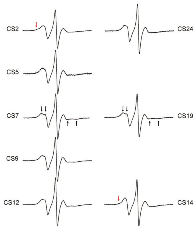
Figure 5. EPR spectra of R5a labeled CS DNA duplexes. Black arrows indicate the resolved hyperfine extrema at CS7 and CS19. Red arrows indicate the presence of a second spectral component at CS2 and CS14. Spectra of CS9, 12, 14, 19, and 24 were corrected for the residual free nitroxide (<3%).
