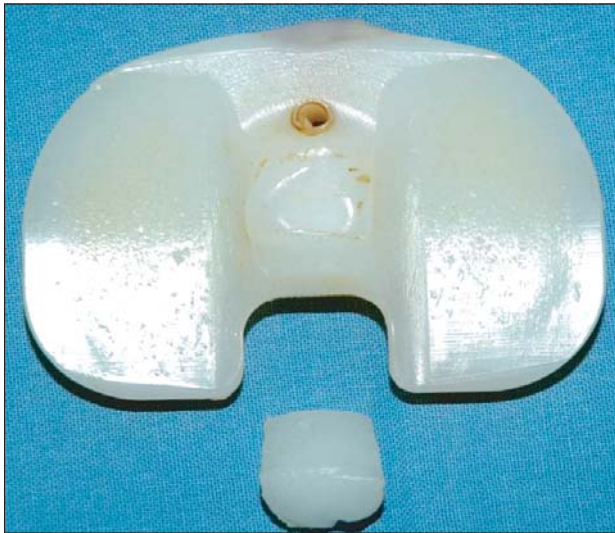
Fig. 4. A photograph of the retrieved insert showing fracture of the poly-ethylene tibial post at its base.
