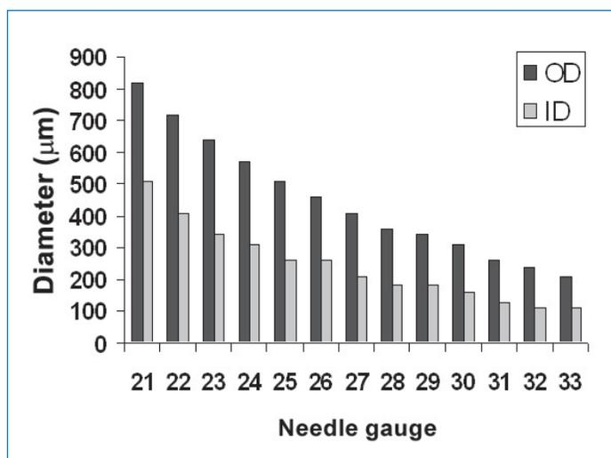
**Figure 2.** Outer and inner diameters of conventional hypodermic needles as a function of needle gauge.
