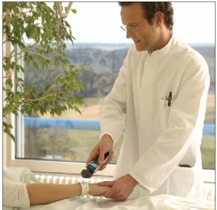
Figure 1. Use of an RFID reader to identify a patient. The RFID tag is on the wristband of the patient. This figure is courtesy of HealthTech Wire/Grundig Business Systems.
