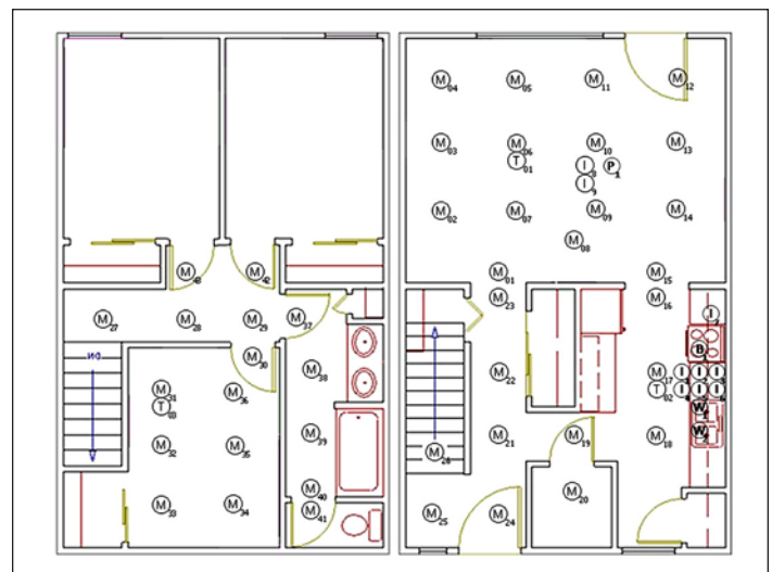
Figure 3. The CASAS apartment. Circles indicate the positions of motion (M), temperature (T), and item (I) sensors throughout the environment.
