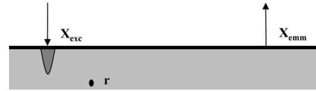
FIG. 1. Semi-infinite tissue model with the excitation and emission fibers on the top surface. The light gray area is the tissue and the dark gray area represents the excitation volume, which is small when the absorption coefficient at the excitation wavelength is large. r is an arbitrary location inside the tissue model.
