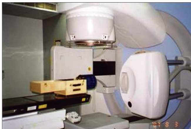
Figure 1: Catphan phantom 503-setup in Linear accelerator
