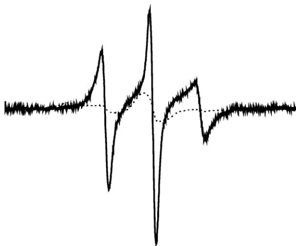
Figure 5. Spectral overlay of Q333R1 (dotted line) and Y408F/Q333R1 (solid line) after correction from the background labeling (the cys-less spectra was subtracted in a one-to-one ratio and using the non normalized spectra). The normalized spectra are shown.
