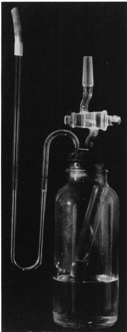
FIG. 1. Gas-collecting apparatus, equipped with mercury manometer to indicate gas pressure and tapered joint to fit the inlet port of the mass spectrometer. Inside the culture bottle is a tube containing 20% KOH to absorb \text{CO}_2 . The inoculum was introduced by syringe through a serum stopper, and the bottle was flushed with argon.
