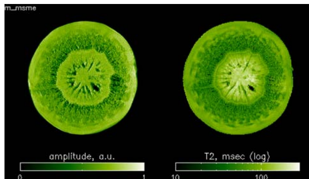
Fig. 2 Amplitude and T_2 map as a result of a MSE experiment on a carrot tap root on a 3 T (128 MHz) MRI system. FOV 40 \times 40 mm, 256 \times 256 image matrix, slice thickness 2 mm: pixel dimension 156 \times 156 \times 2,000 \mu m^3
