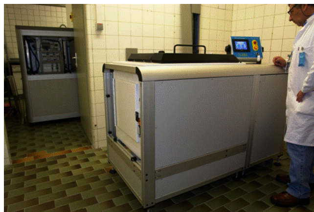
Figure 2 Prototype X ray machine. An RS2400 self-shielded cabinet 150 kV X ray irradiator (Rad Source Technologies Inc, Alpharetta, Georgia, USA), with a working volume of about 18 L divided into 5 horizontal cylinders 176 mm diameter by 150 mm long (3.6 L each) with a dose uniformity ratio of 1.3. This unit requires a 10 kW, three phase electrical supply and is cooled by chilled water or a self contained water-to-air heat exchanger (seen in the background). High power X ray units have only recently become available and are not in general use yet.
