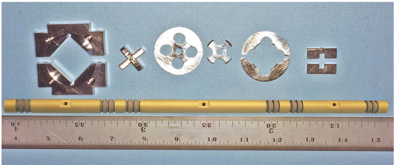
Fig. 3. Photograph of the electrostatic lens components (L to R): V-blocks used to clamp the lens rods; assembled cross spacer; field shaping disc; inner (cross) and outer (ring) parts of the field shaping disc; and two halves of a cross spacer. Below these components is one of the ceramic rods for a quadrupole triplet.
