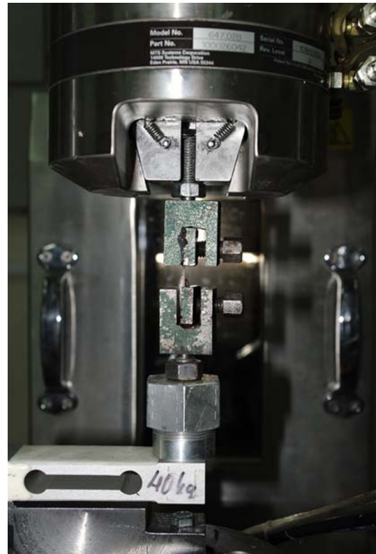
Fig. 2 Biomechanical test machine (MTS 858 MiniBionix II Axial Torsional Testing Machine [S/N:10189576])
