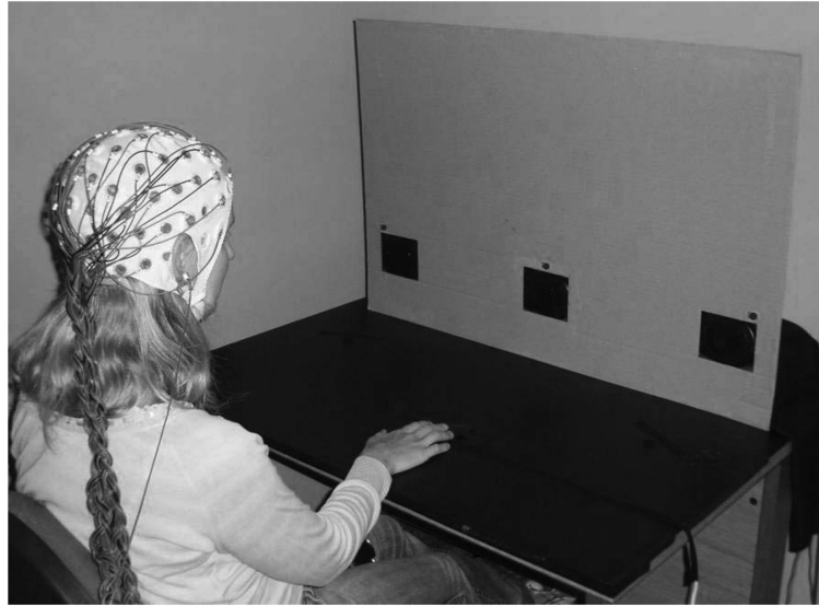
Figure 1. Stimulus setup used in this study. Sounds were presented from any one of three loudspeakers. The squares located above each loudspeaker indicate the fixation point (above the central loudspeaker) or the goal locations for leftward or rightward saccades (above the left and right loudspeakers). Response keys were aligned with the central loudspeaker.
