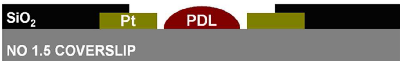
Figure 2. Schematic of the surface patterning of poly-D-lysine (PDL) on the platinum (Pt) electrode arrays before (a) and after (b) dry lift-off.
