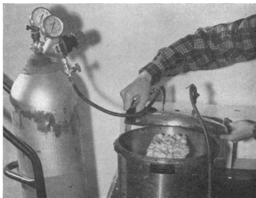
FIG. 1. Modified pressure cooker used as an anaerobic chamber.
