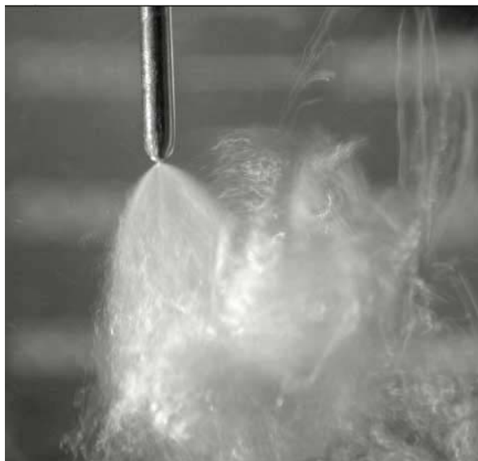
Figure 3. Spray profile for a \text{CO}_2 solution expanding through a tapered elliptical nozzle with a flow rate of 2.5 mL/min at 345 bar.
