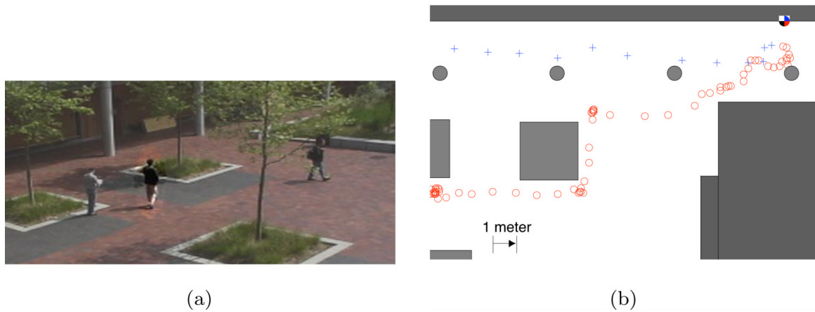
Fig. 4. (color online) (a) The E2 courtyard where the outdoor tests took place. Highlighted is subject D during one of the sessions. (b) Blueprint of a portion of the E2 courtyard. Non-accessible grey areas indicate pillars, walls, or grass patches. Two partial trajectories leading to the color marker are shown via blue crosses (subject B) and red circles (subject D). Each mark corresponds to the location of the subject measured every 0.5 seconds.
