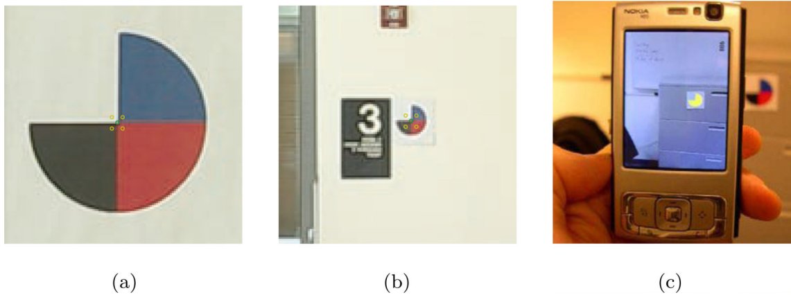
Fig. 1. (color online) (a), (b): Our color marker seen at a distance of 1 meter and of 6 meters respectively. The figures shows a 121 \times 121 pixel subimage cropped from the original 640 \times 480 pixel image. Superimposed are the locations of the 4 pixels of a “probe” placed at the center of the marker's image. Note the probe's size is the same for the two images, and that correct detection is attained in both cases. (c): The color marker region is segmented (shown in yellow) after detection.
