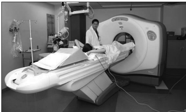
Figure 5) The figure shows the new, noninvasive, 64-slice fast computed tomography scanner for performing coronary angiograms. It requires approximately 45 s to image the coronary arteries and a total time of approximately 20 min from entry of the patient until completion. This makes it possible to perform coronary angiograms on asymptomatic control subjects
