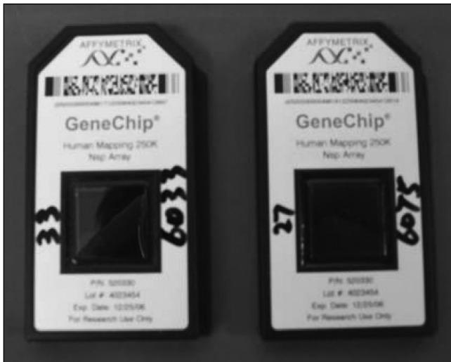
Figure 1) The Affymetrix GeneChip Human Mapping 500K Array Set (Affymetrix Inc, USA). Each chip comprises 250,000 single nucleotide polymorphisms (SNPs), and together, they comprise the 500,000 SNPs that scan the human genome at an interval of 6000 base pairs
