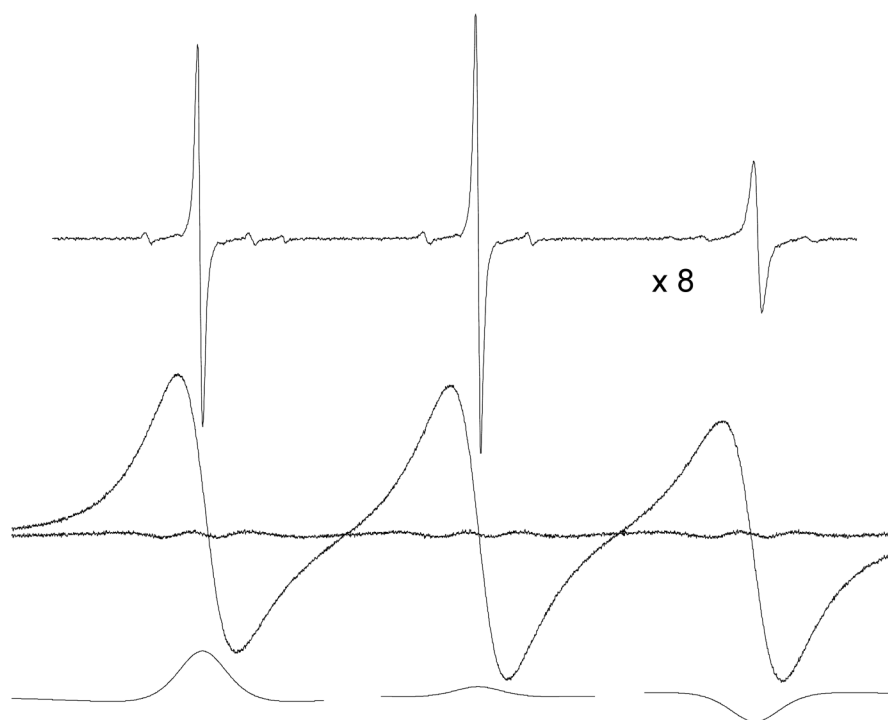
Figure 2. EPR spectra due to 0.1 (top trace, at a relative gain of \times 8 ) and 93.6 mM (middle trace) PDT in 70% glycerol at 293 K. The fit and spectrum are indistinguishable; however, a definite residual is evident due to a significant dipolar interaction; the fractional broadening by spin exchange is \Omega(T) = 0.30 \pm 0.03 .
