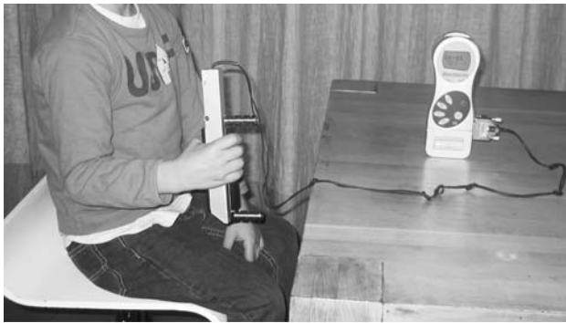
Fig. 1 A 6-year-old child holds a Jamar-like dynamometer (Lode dynamometer). The electronic console was facing the researcher so that no feedback was provided to the subjects.
