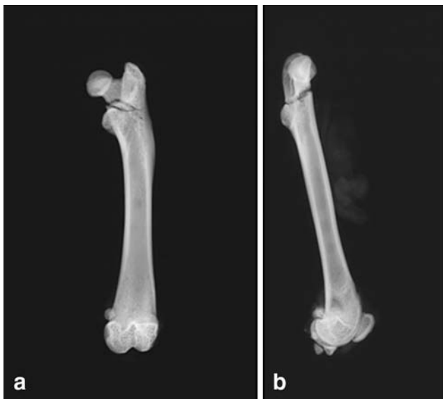
Fig. 4 Radiographs of proximal rat femur after breaking test. We observed in 86.6% of cases (in right–left comparison) a reverse trochanteric fracture (type A 3 according to AO classification; a anterior–posterior view, b lateral view)
