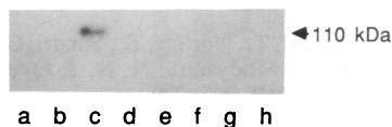
FIG. 5. Phosphorylation of a 110-kDa protein band in microsomal fractions from COS-1 cells transfected with wild-type and mutant cDNAs encoding the Ca 2+ -ATPase. Membrane proteins were phosphorylated with [ \gamma - 32 P]ATP, separated on a polyacrylamide gel, and subjected to autoradiography. Nontransfected cells in the presence (lane a) and absence (lane b) of Ca 2+ ; wild-type cDNA in the presence (lane c) and absence (lane d) of Ca 2+ ; and mutants aspartic acid-351 to glutamic acid (lane e), asparagine (lane f), threonine (lane g), and alanine (lane h) in the presence of Ca 2+ .
