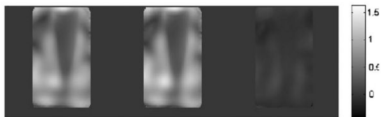
Figure 8. The motion amplitude estimated from 32 (left) and 3 (middle) phase offsets; the right image is the difference between the former two images.
