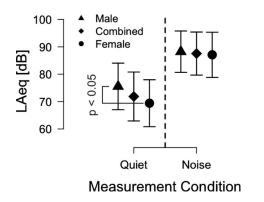
FIG. 5. Mean  $L_{Aeq}$  values in quiet (left) and in noise (right) for the entire subject pool and those for the male and female subjects. The error bars represent  $\pm 1$  standard deviation.
