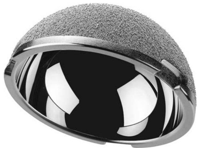
Fig. 1 A photograph shows the Conserve Plus ® acetabular component (3.7-mm wall thickness) with porous beaded surface made of cobalt-chrome molybdenum alloy for osteointegration without supplemental screw fixation.
