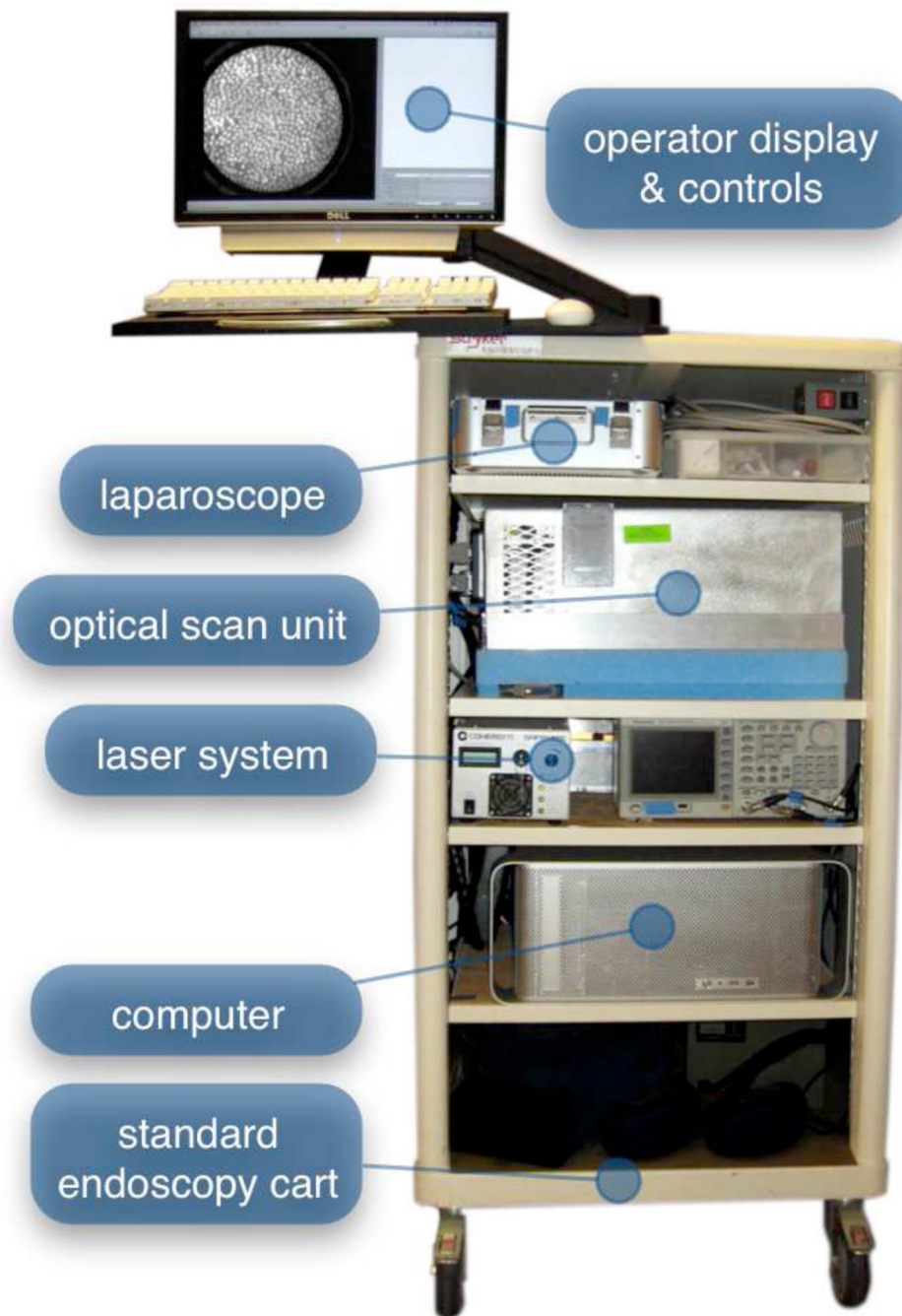
Figure 2. The mobile cart. Shelves on the cart, from top to bottom, contain the sterilized microlaparoscope, optical scan unit, laser power supply and system electronics, and computer. The top of the cart holds the operator controls and the primary display.
