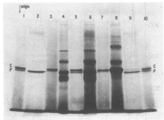
FIG. 8. Electrophoresis of various ET preparations on a 12.5% SDS-polyacrylamide slab gel. The gel channels were loaded with either 70 to 100 \mu g of purified, electrofocused ET protein or 375 \mu g of partially purified toxin preparations (crude) obtained after (NH 4 ) 2 SO 4 precipitation. Electrophoresis was carried out with constant voltage and a current of 35 mA until the front of the dye marker reached the bottom of the gel. C marks the bands of ET regulated by a chromosomal genetic determinant, and P marks the bands of ET regulated by a genetic determinant on the 56S virulence plasmid. (1) Electrofocused ET from strain UT0002; (2) electrofocused ET from strain UT0007; (3) electrofocused ET from strain UT0002-19; (4) crude preparation of ET from strain UT0007; (5) electrofocused ET from strain UT0002; (6) crude preparation of ET from strain UT0007; (7) electrofocused ET from strain UT0002-19; (8) crude preparation of ET from strain UT0002-19; (9) electrofocused ET from strain UT0002-19 mixed with electrofocused ET from strain UT0007; (10) electrofocused ET from strain UT0002. (Photograph provided by Bill B. Wiley and reproduced from reference 185.)
