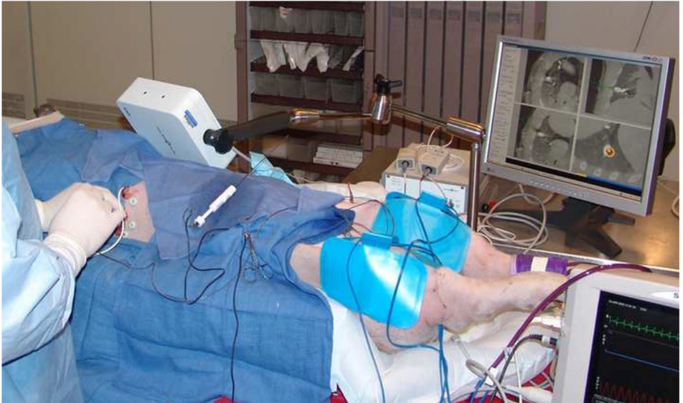
Figure 5. The electromagnetic field generator is shown above the anesthetized animal as it would be positioned during a typical experimental setup. The user is advancing an EM tracked trocar/stylet into the pre-planned target using only the graphical user interface (top right) without real-time imaging.
