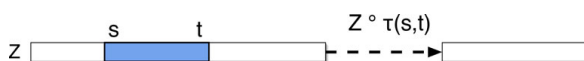
Figure 6 A delete operation. A delete operation, denoted \tau(s, t) . The substring z_s, \dots, z_t is deleted.
