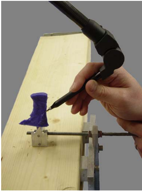
Figure 2 Reattachment of the cast of the carpal tunnel to the apparatus for digitization of its surface.
