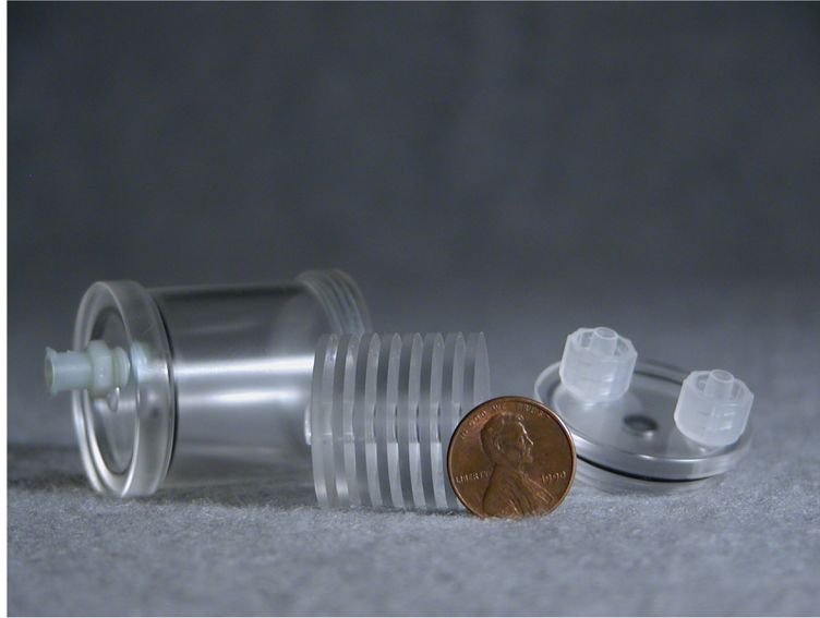
Figure 2. Ultra Micro Cold-Disk Phantom. The disks and spacing are 1.6 mm thick and 22 mm in diameter.
