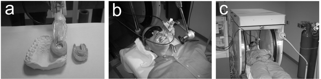
Fig. 2. During in vivo tooth dosimetry measurements: (a) the resonator is held in proper position using a custom-made mold, (b) the mold and resonator are placed in the oral cavity over the teeth of interest, along with absorptive pads to sequester saliva, and (c) the patient bed is inserted into the magnet for measurement with the teeth centered with respect to the magnet and modulation coils.
