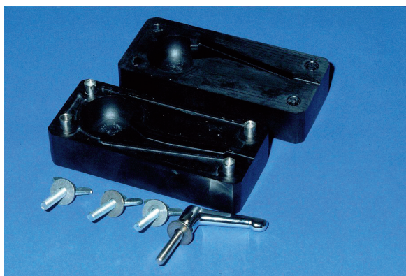
Figure 1. Mold, consisting of polyoxymethylene (POM), for standardized production of hip spacers. Each spacer has a head diameter of 50 mm, a stem length of 10 cm, and a total surface area of 13,300 mm 2 .
