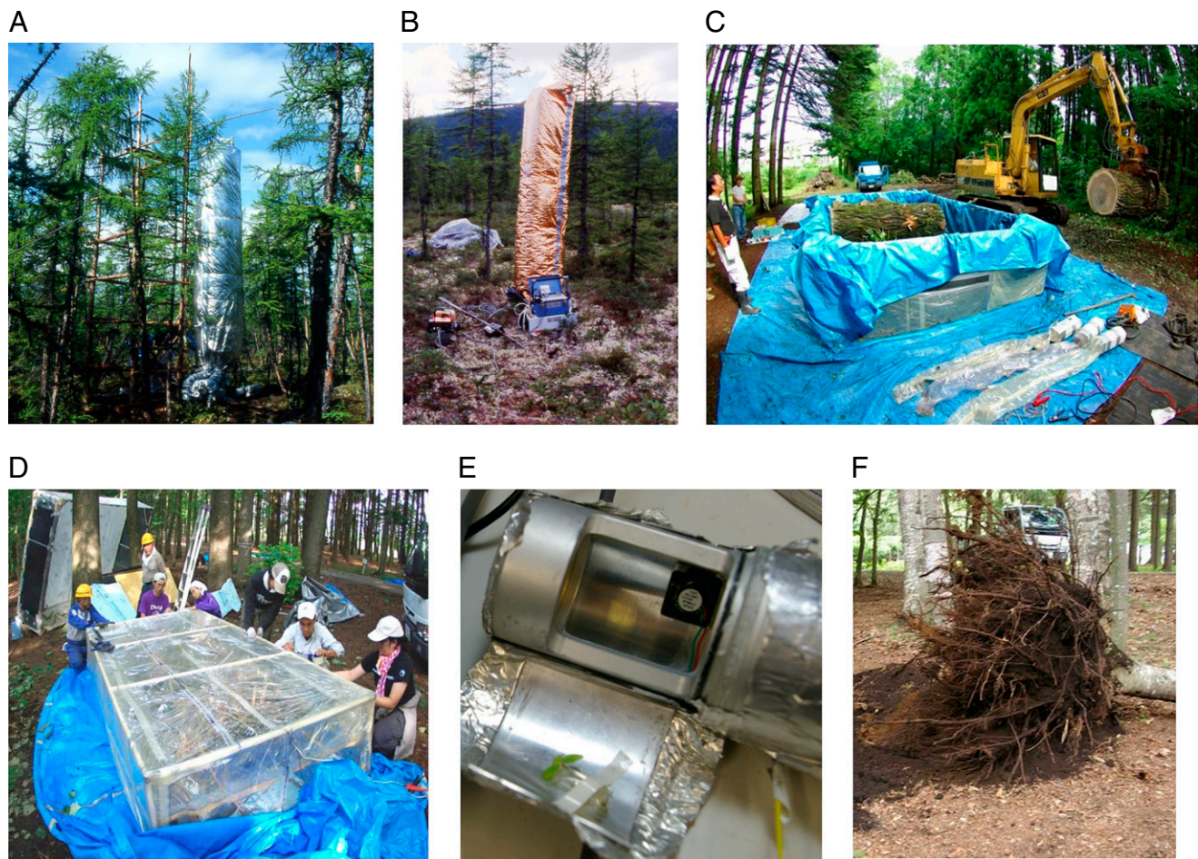
Fig. 1. Our methods for measuring whole-plant respiration from seedlings to giant trees using closed-air circulation chamber for all sample plants. (A) Measurement of a standing tree using a dark chamber in Siberia, with air temperature controlled using heat generated from wood fires and permafrost (as schematic representation of the system in Fig. S2, and as exemplification of measured data in Fig. S3). (B) Measurement of a standing tree using a dark chamber in Siberia without an air-temperature controller. (C) Measurement of excised and excavated materials from a large tree using a destructive method. (D) Measurement of excised and excavated materials from a midsize tree using a destructive method. (E) Measurement of excised or excavated seedlings. (F) The roots of midsize trees immediately after rapid excavation.
