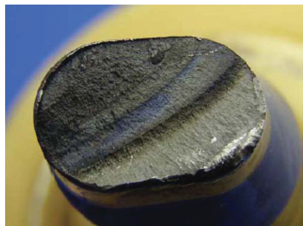
Figure 8 Fatigue fracture surface of a clinically failed titanium neck adapter.
