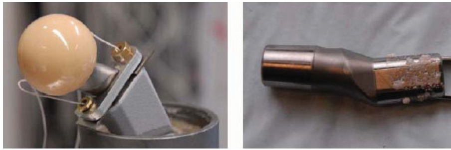
Figure 6 Test setup for measurement of micromotions in the modular cone connection (left) and particle-contaminated joining area (right) [18,19].
