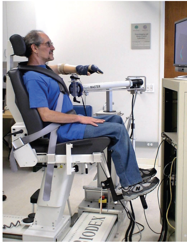
Figure 1. Participant seated in the Arm Coordination Training 3D device (ACT 3D ) system. Straps secure his trunk, and the arm is attached via a lightweight splint. He is looking at the computer monitor for visual feedback.
